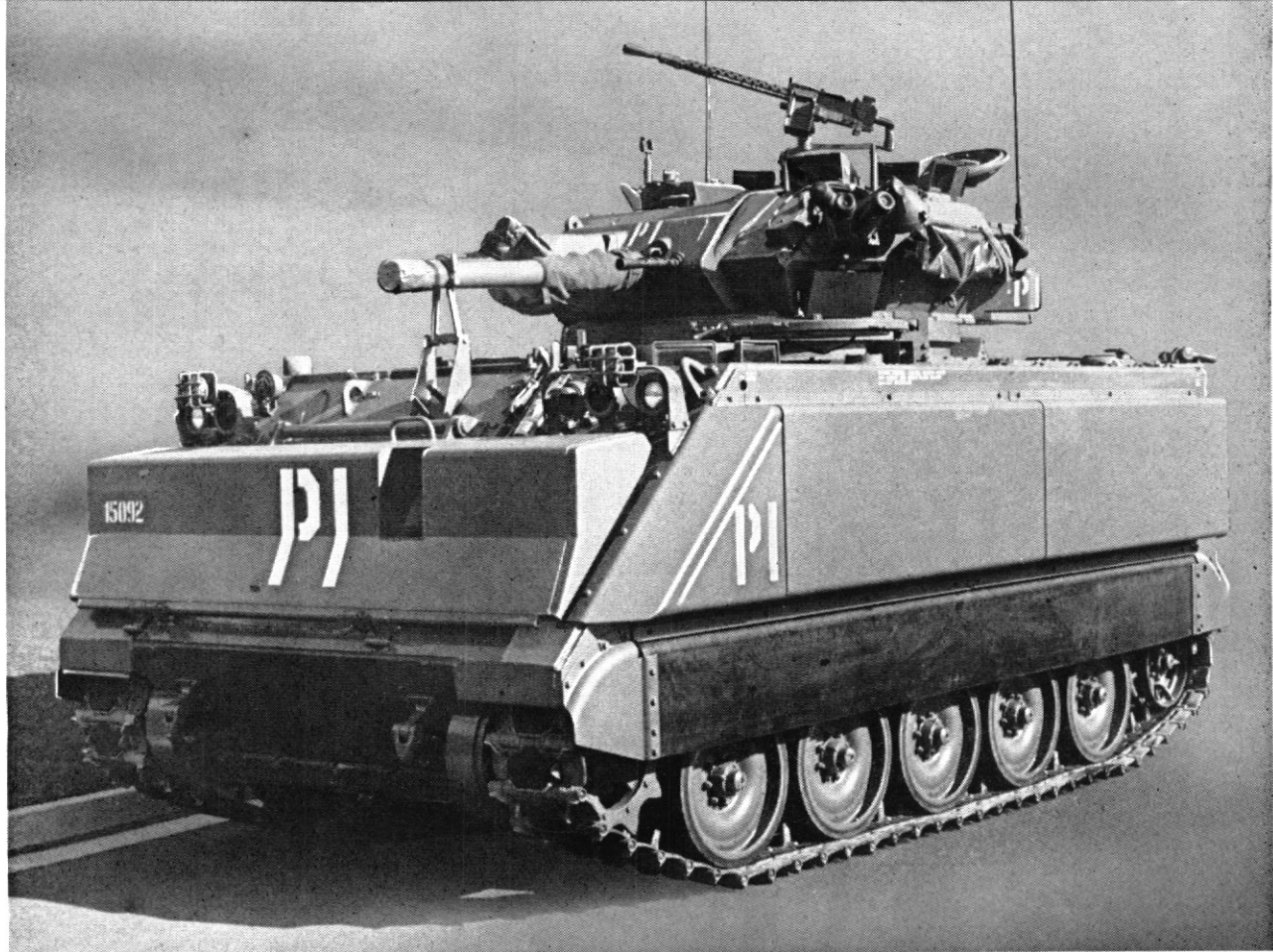
The Army's new Fire Support Vehicle. This ESV is basically an M113A1 armoured personnel carrier to which a British
