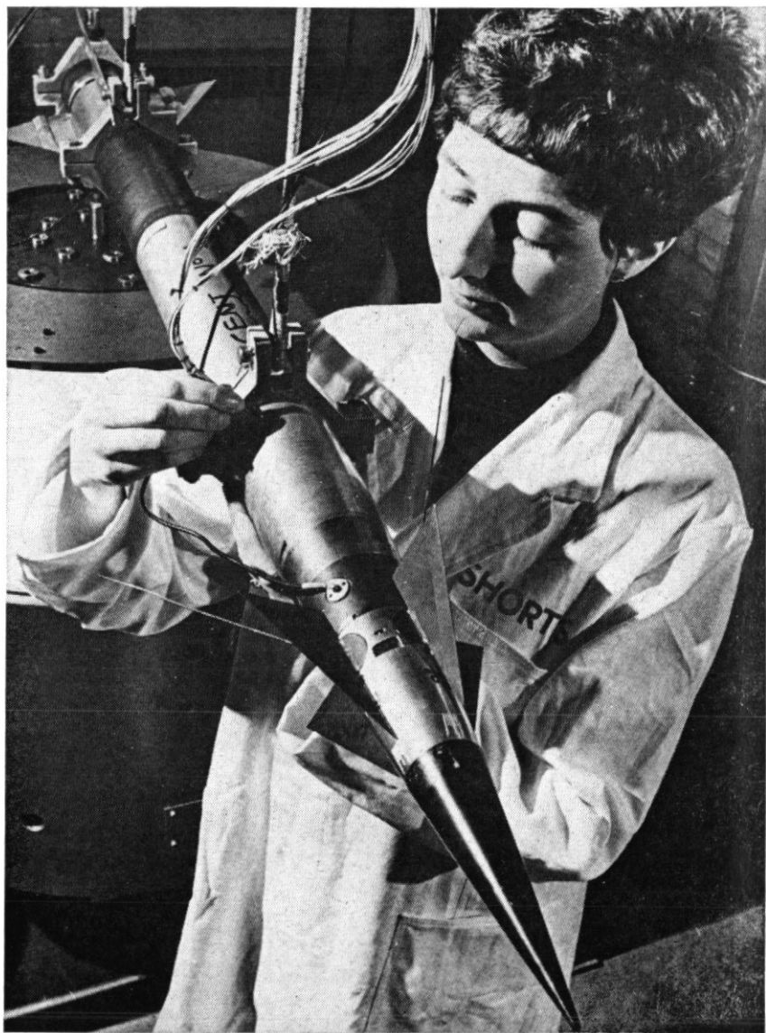
A Blowpipe missile, showing the slender nose with its guidance vanes and the receiver aerials and other features.
