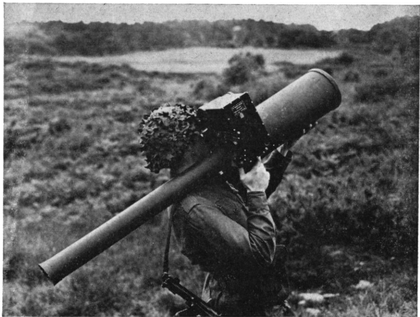
A soldier aiming Blowpipe. His right hand is holding the grip with his thumb on the guidance button.
