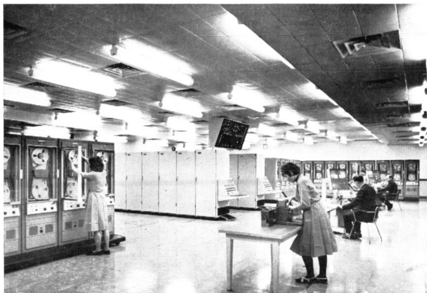
RAF AEI 1010. General view showing magnetic tape units, console and display unit
