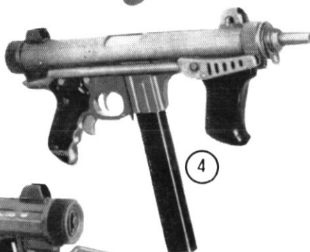
4 & 5. Beretta (Italy) 9mm with stock folded and extended Note cocking handle and hooded foresight.
