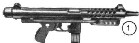
1 Star (Spain) 9mm with stock in folded position. Note cocking handle folded above magazine and double notched trigger, top half being for fully automatic fire.
