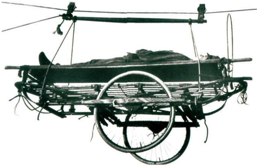
A portable stretcher and carriage, designed by Sergeant Worsfold, 9th Australian Field Ambulance, with special attachment for hauling along aerial line.
