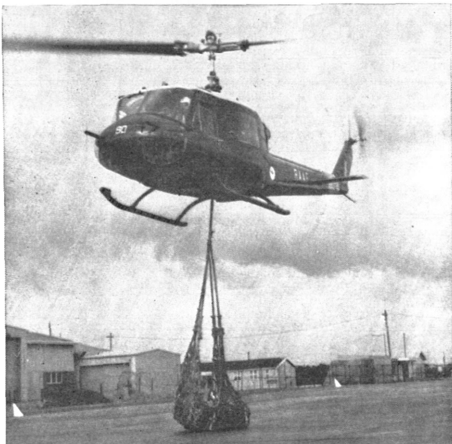
An Iroquois helicopter employing the under-slung load technique.
