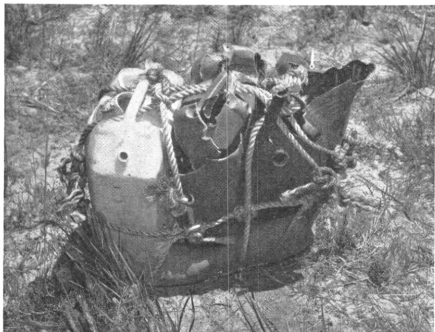
Picture illustrates the damage caused by overfilled plastic water containers which were air-dropped.—Army P.R. Photo.
