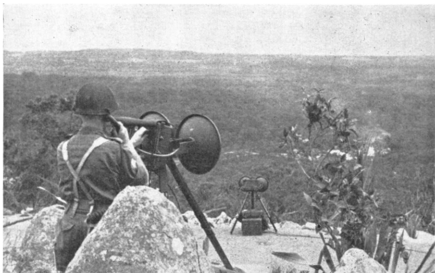
A WS B70 repeater station (Telegraph Hill).
