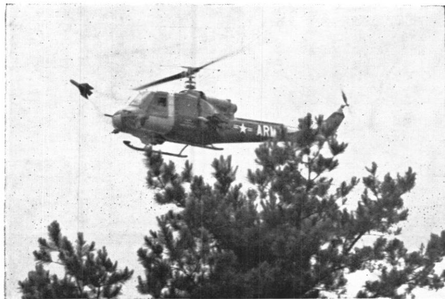
The UH1 launches an SSII anti-tank guided missile.
