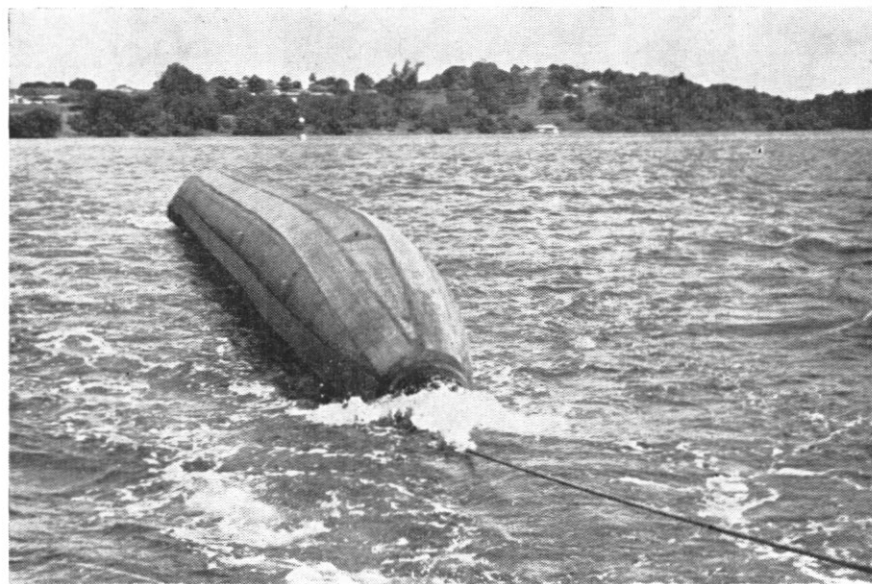
Empty Dracone being towed on short wire, nose cone making bow wave.
