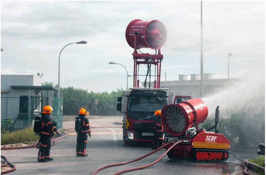
Figure 7: SCDF's Ventilation Vehicle (left) introducing water mist to disperse chemical vapours during Exercise Northstar XI. The Unmanned Firefighting Machine (right) provides SCDF with sustained fire suppression capabilities and frees up frontliners to focus on other critical aspects of the operation. Source: SCDF.
