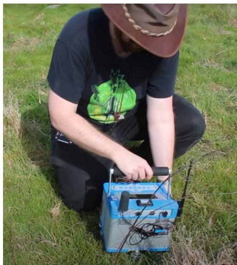
Figure 3: Operating a GC-6 gravimeter in the field. RTK GPS is attached to the back of the device.
