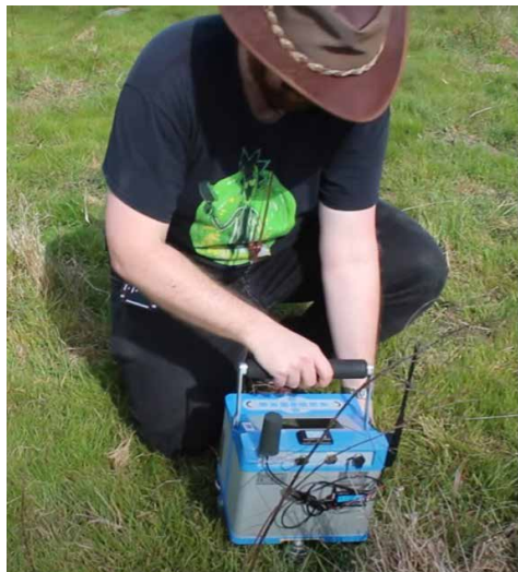
Figure 3: Operating a CG6 gravimeter in the field. RTK GPS is attached to the back of the device.
