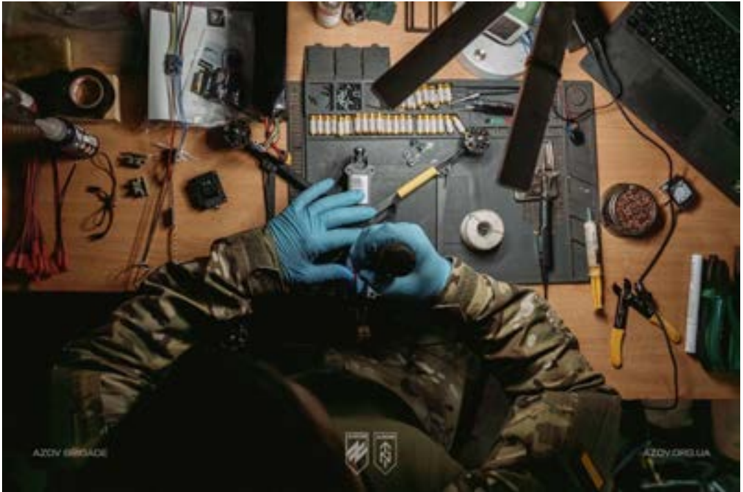
Figure 40. Building an FPV drone from components in the workshop. Photo Credit: 12th Special Operations Forces Brigade Azov, First Corps Azov of the National Guard of Ukraine. Photo reproduced with the owner's permission.
