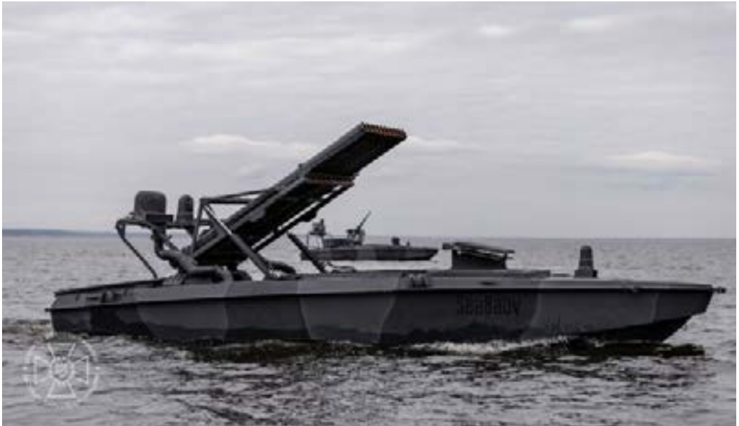
Figure 20. Ukrainian Sea Baby naval drone with a 122 mm rocket launcher. October 2025. Photo credit SSU. Obtained from Militarnyi SSU Presents New Generation of Sea Baby Naval Drones: Range Exceeds 1,500 km 61
