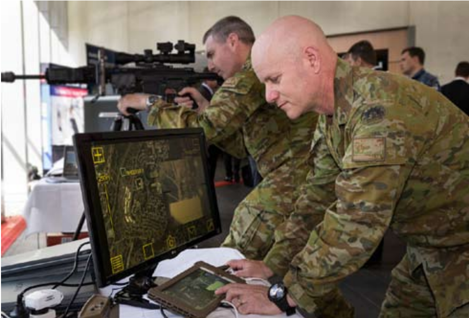
Figure 28. Two Army officers test the Sword sniper system. The Sniper Weapon and Observer Reconnaissance Devices are networked weapons targeting systems that integrate cameras, GPS rangefinders, Android mobile apps and other components which allows multiple snipers and other viewers to see what the shooter and observer are seeing so that targets can be coordinated and prosecuted. (Image: DoD)
