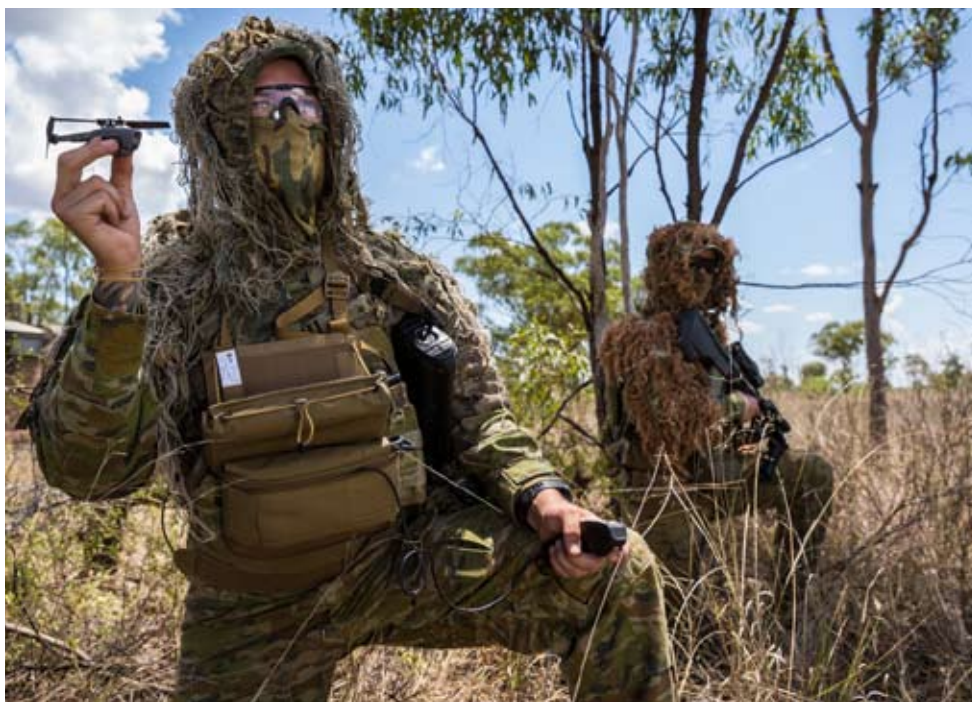
Figure 35. A soldier from 3rd Brigade launches a PD-100 Black Hornet Nano unmanned aerial vehicle. The Black Hornet is a simple UAS able to provide short-range reconnaissance and is virtually undetectable when flying a mere 10 metres above the enemy. (Image: DoD)
