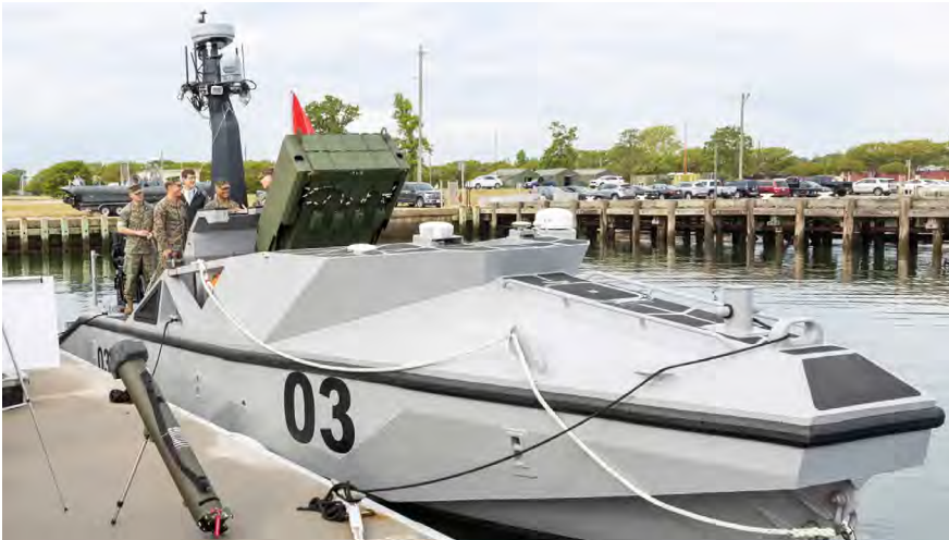
Figure 5. Long- Range Unmanned Surface Vessel with Multi-Canister Launcher (Source: Defense Visual Information Distribution Service) 60
