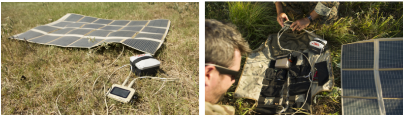
Image 5: In field battery charging solution for squad UAV by Aeryon Labs Inc.
