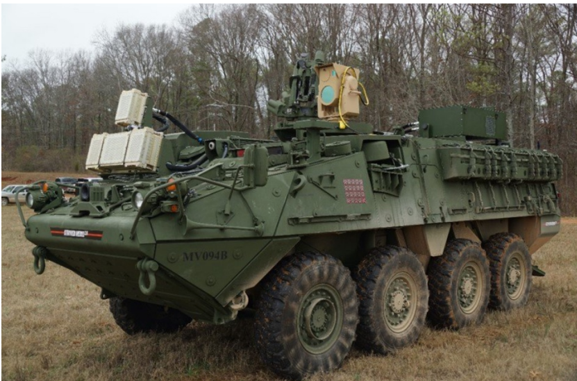
Image 4: The US Army is developing Manoeuvre Short-Range Air defence capabilities based on the Stryker Anti-aircraft variant. Future evolutions of this capability will demand in excess of 100 KW of electrical power which is currently not achievable with conventional propulsion systems.
