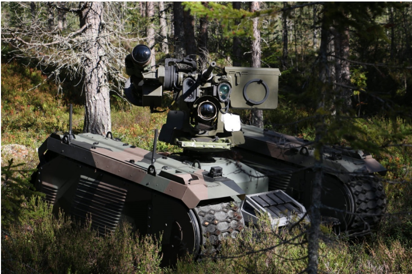
Image 6: Milrem Robotics Tracked Hybrid Modular Infantry System (THeMIS) supports dismounted troops through various sub-system configurations and is a potential energy source for dismounted combatants. Photo courtesy of Milrem Robotics
