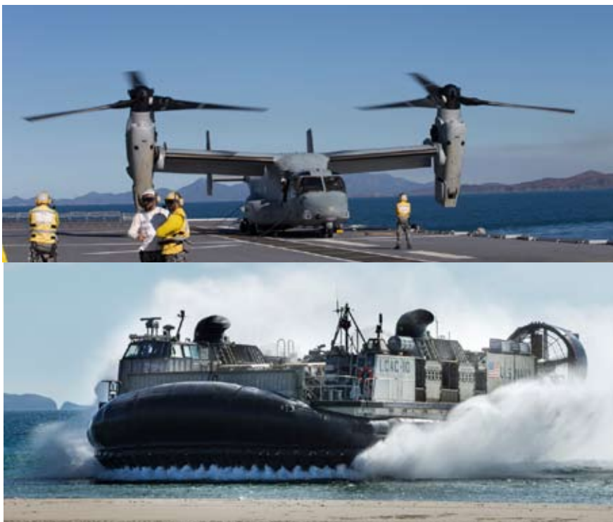
Figures 6 and 7. An MV-22 Osprey of the USMC on board HMAS Canberra as part of a joint combined exercise and (below), a US Landing Craft Air Cushion (LCAC) which can take personnel and equipment rapidly from ship to shore and deposit them directly onto the upper parts of the beach. (Images: DoD)
