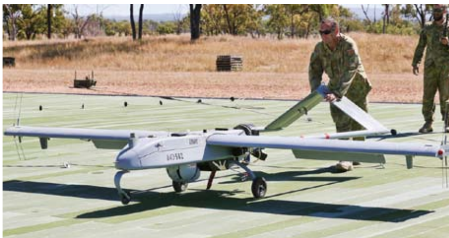
Figure 22. The RQ-7 Shadow as used by both the Australian Army and the US Marine Corps. This unmanned aircraft uses a noisy rotary engine which can be used as part of a deception plan. (Image: DoD)
