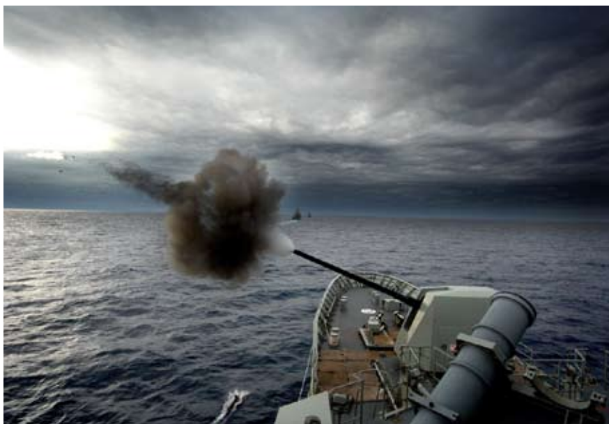
Figure 17. HMAS Warramunga fires its 5 inch guns. This type of gun has a range of 24 km and can fire at a maximum rate of 16 - 20 rounds per minute. This class of ship carries up to 680 rounds.
